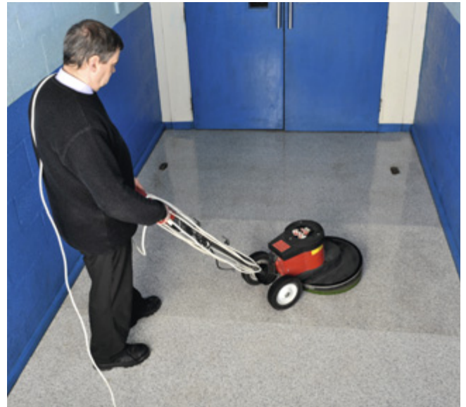
Floor area cleaned with machine scrubber and green pad
