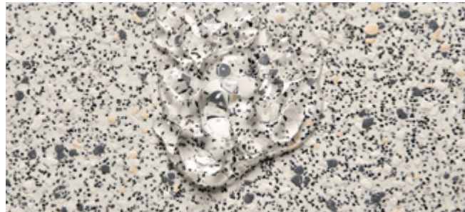
Polysafe Corona PUR with commonly used alco-based hand gel applied to the surface.
